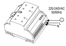
Figure 2: ZPS640HIC230 installation and connection
